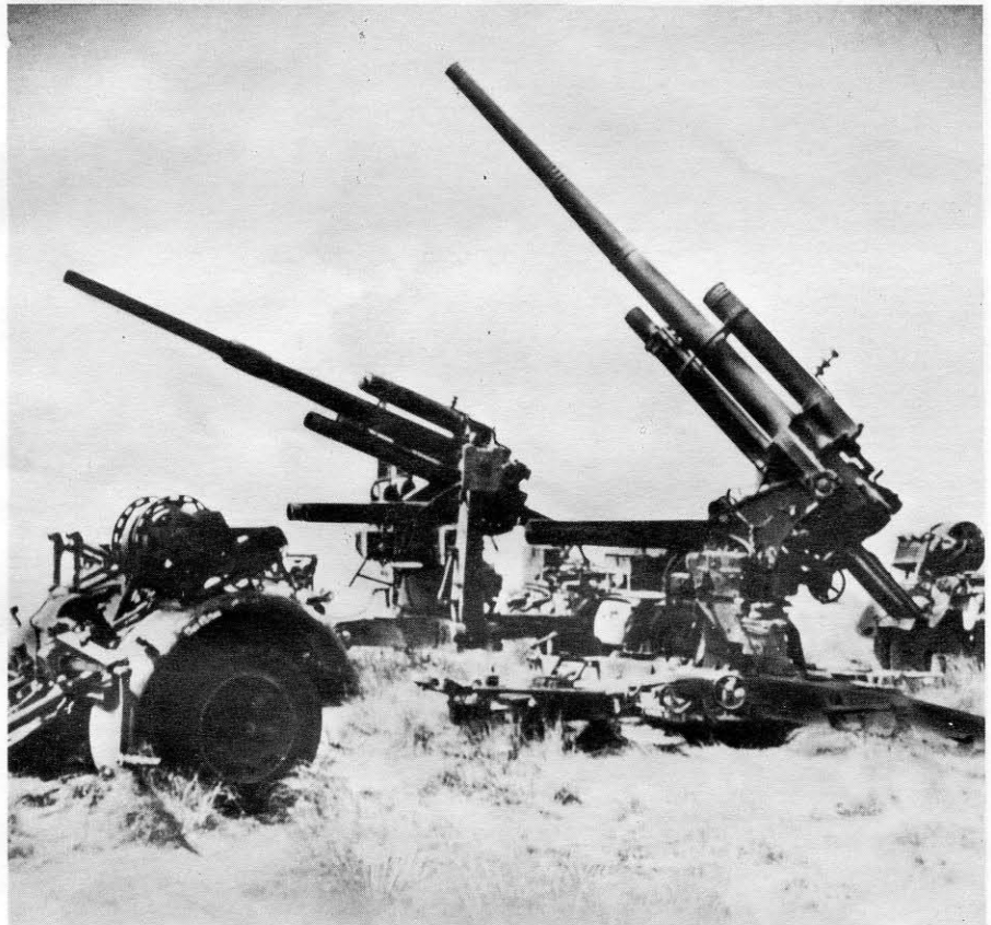
Flak 18 (Right) and Flak 36 (Left), Note the difference of Barrel
